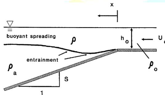
Figure 22. Buoyant surface discharge on a sloping surface.
