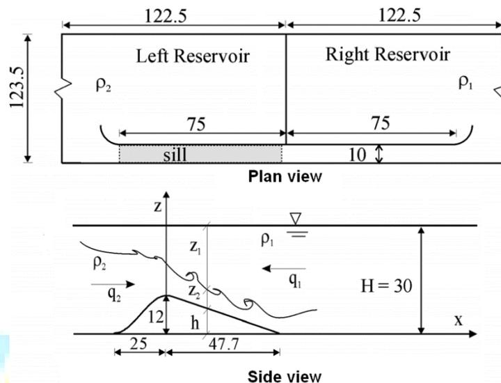
Figure 25. Schematic of the experimental set-up [29].
