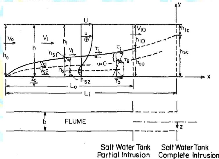
Figure 16. Sketch of the arrested salt wedge [19].
