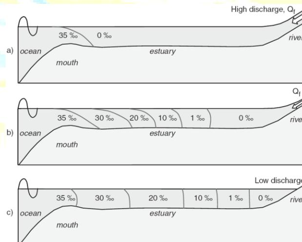
Figure 10. Salinity for (a) a stratified, (b) a partially mixed, and (c) a well-mixed estuary [2].
