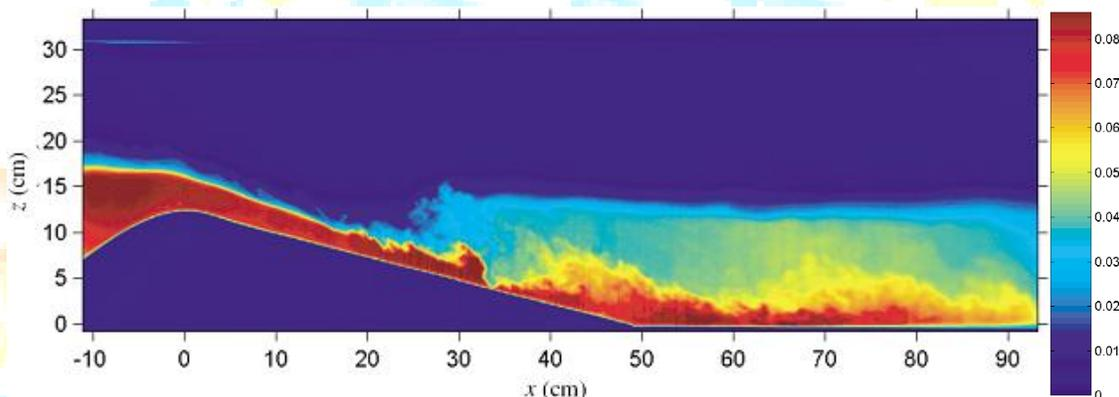
Figure 26. Time-averaged concentration profiles. The scale indicates concentration levels in  $\mu\text{g/L}$  [29].
