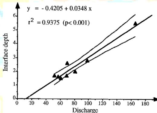
Figure 14. Regression of river discharge ( $\text{m}^3/\text{s}$ ) vs. interface depth (m) Ibanez et al. [14].
